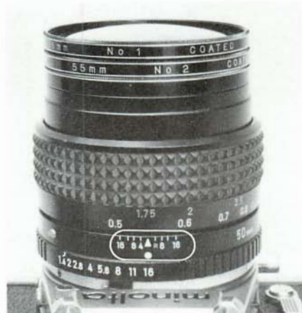
3 – A typical depth-of-field scale on a SLR lens.
