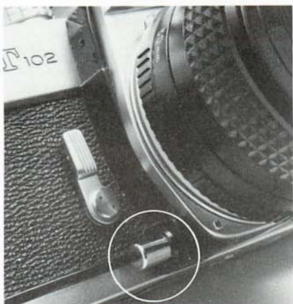
1 – A typical depth-of-field preview button on a SLR camera body.
