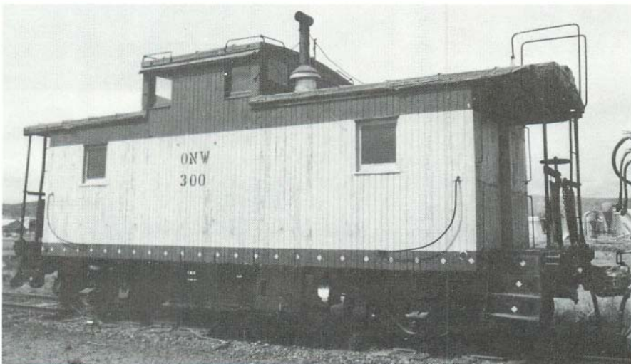
O&NW 300 before removal of roof handrails above ladder. Photo shows placement of relocated stove vent and added propane tank and battery box.
