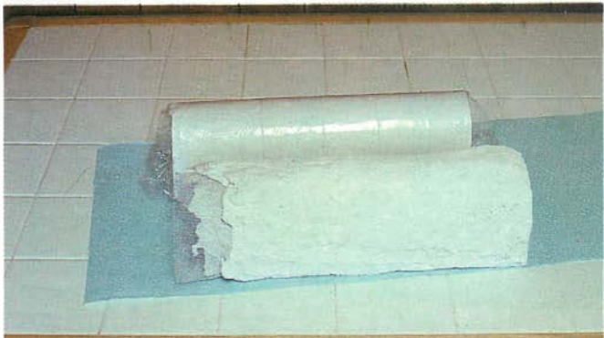
5 – The Jersey Western tunnel lining was cast using a homemade mold that had seams representing the separate sections of the prototype tunnel.
