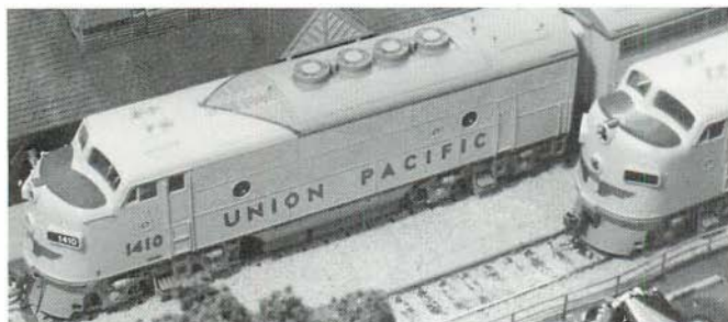
Stewart F3A (top track) after detailing with Detail Associates DK701 kit and other detail parts.
