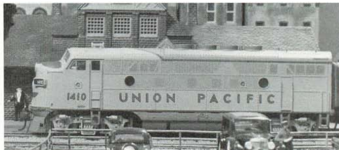
Side view highlights multi-depth casting which shows vents, frame and car side under chicken-wire detail.
