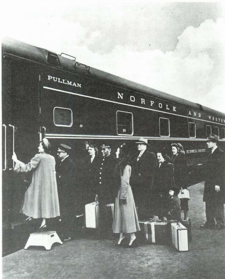
Pullman Standard delivered three class S2 sleepers in December 1948. Each had a ten-roomette/six-bedroom arrangement and rode on T-96 trucks. Cost was $119,290 each.
