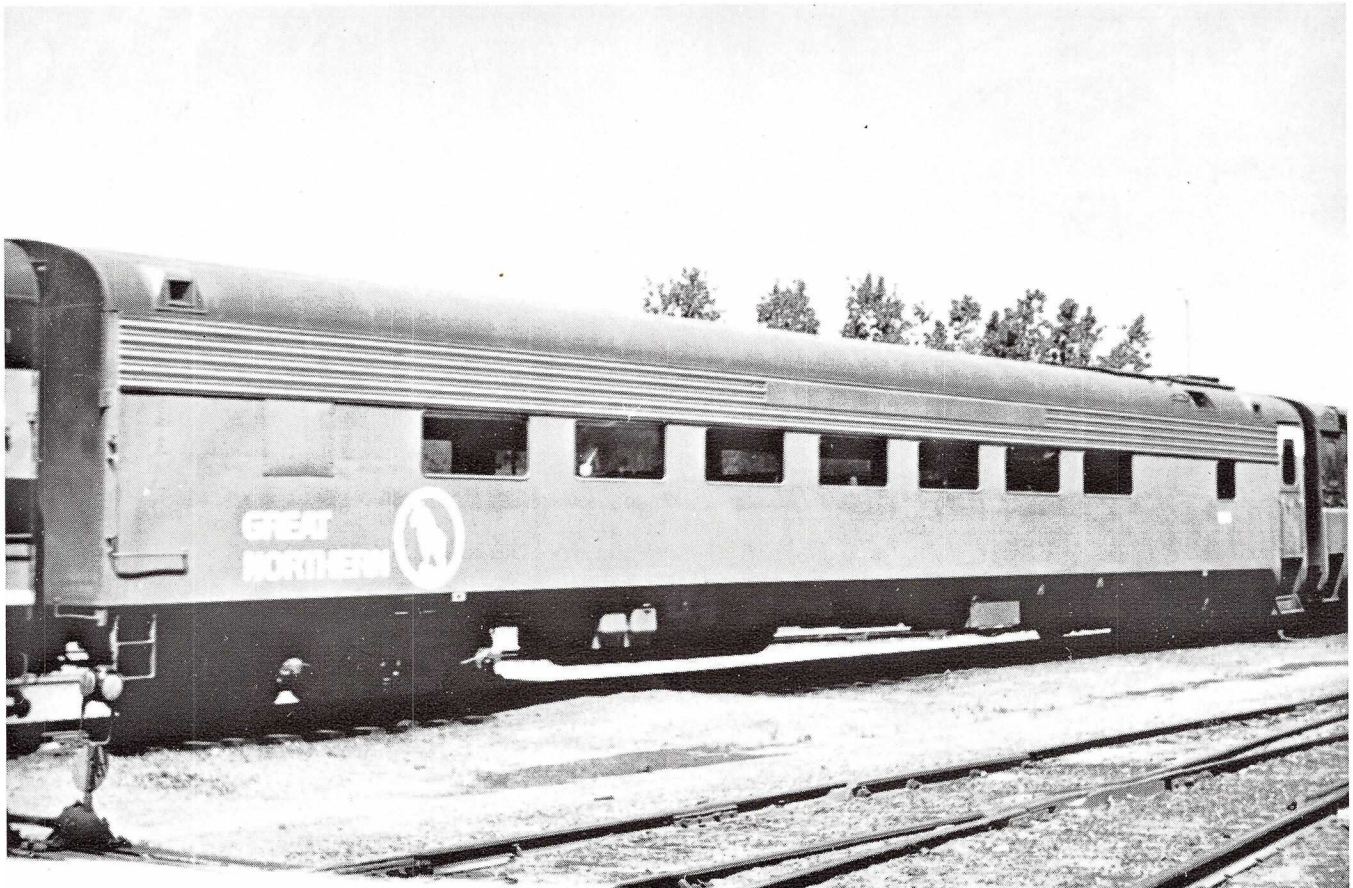
The unmistakable appearance of car No. 1074 (corrugated sheathing above the windows and painted flat steel below) was the result of structural repairs in 1969. A window was blanked when the buffet was installed. C.A. Rudisel photo.
