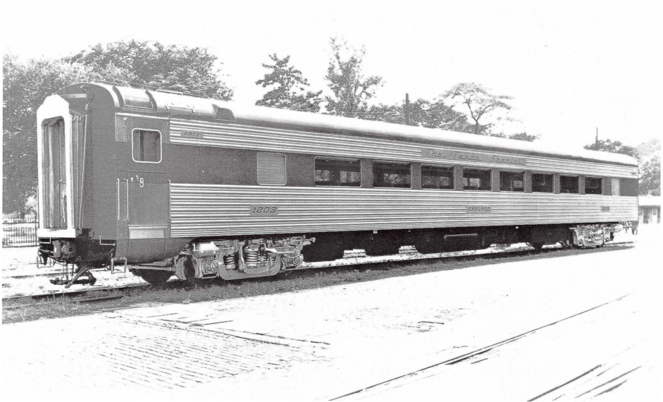
Frisco No. 1259 (GN 1075) was identical to Katy No. 1203 pictured above. These cars were notable for their all-stainless steel body frame construction and Melamine plastic (low maintenance) interior finish. The 1203 became NP 531 in 1966, and later was among 16 former Texas Special and Meteor cars to wind up on the BN, via GN, NP and SP&S. Pullman-Standard photo, W.D. Randall collection.
