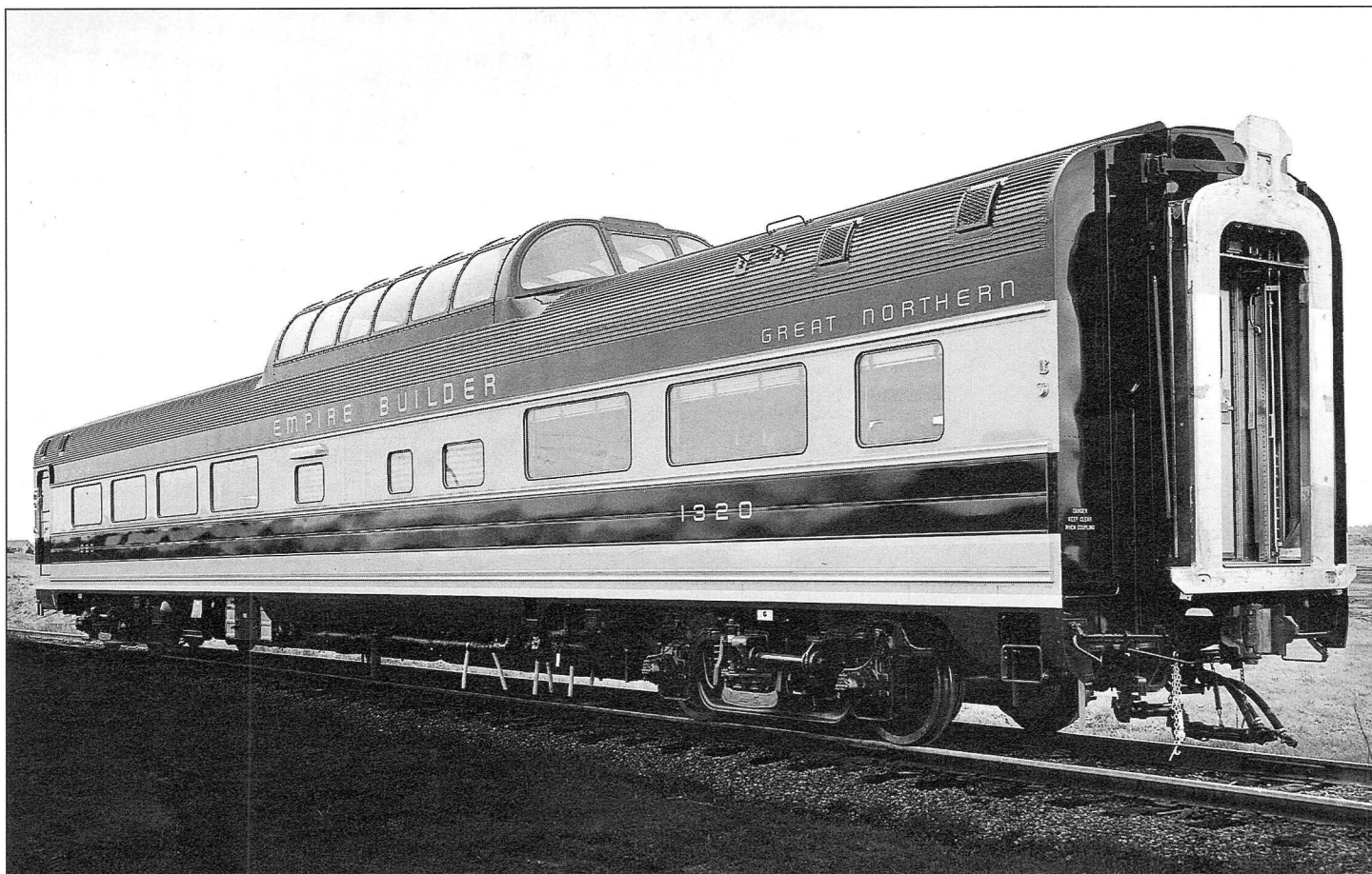
A gleaming, brand new, GN Dome Coach, ready to give 46 coach seats and 24 dome seats to expectant passengers. The three domes usually in the consist replaced the 48 seat coaches of the earlier version of the train. The seats were available to coach class passengers. GNRHS Archives.
