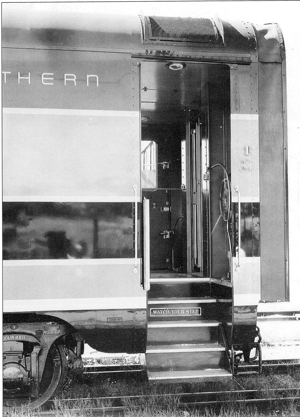
While there are many photographs of the exterior of passenger cars, very few have been published showing the Entry Vestibule of a car. This is what the passenger saw entraining a GN streamliner. A very clean and update design is shown in this GN Archives photograph.
