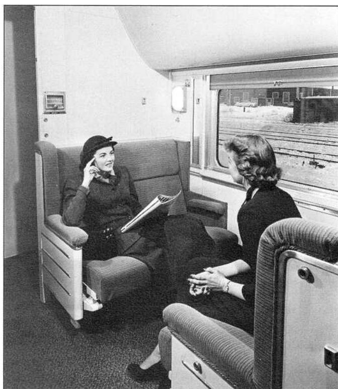
By day, an open section in the sleeping cars has two full seats for its two occupants. At night this space is transformed into a lower and an upper berth. The upper berth is let down from the angle of the upper wall and ceiling by the attendant. Curtains are closed and fastened for privacy.
