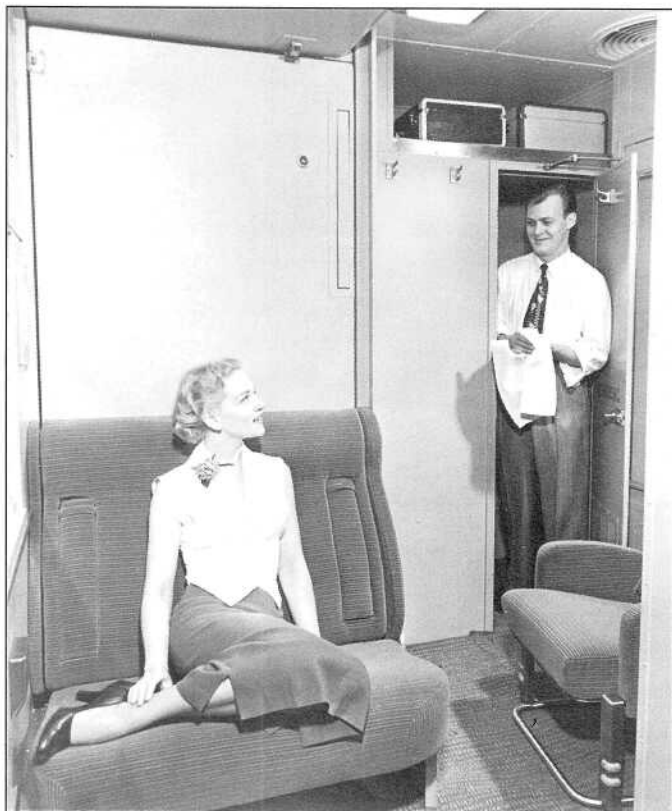
above: A sleeping compartment, larger than a bedroom, is designed for two passengers. The door leads to toilet and lavatory facilities in the annex. At above right, the compartment is shown with its two single beds made up by the attendant. The upper and lower beds are aligned lengthwise within the car, and the exit door to the aisle of the car is out of view to the right of the picture.
