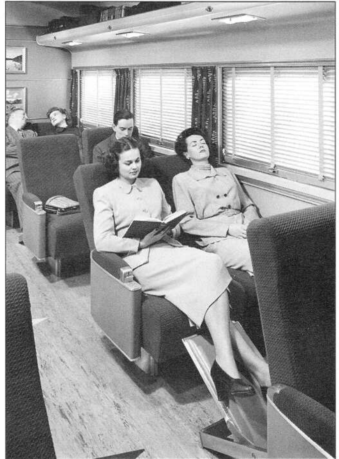
Longer distance coach passengers travel with more space in the 48-seat Day-Nite coaches. Chaise lounge seats are equipped with combination adjustable leg and foot rests.
