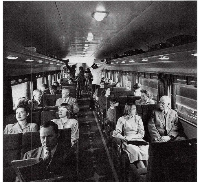
above: full length view of the "shorts" (for short distance passengers). This car had foot rests, and was designed for intermediate station coach travel. The interior color of the "shorts" car was blue.
