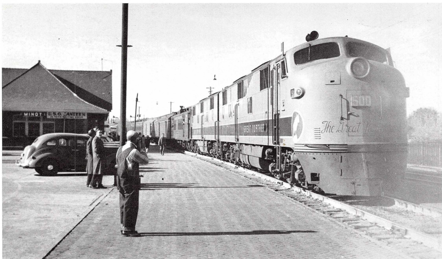
Diesel-electric unit No. 500 A-B on the Second #2, the Empire Builder (1929 consist), arriving Minot, North Dakota. The EMD E7 diesels are brand new, and are in "shakedown" service. Note "The Great Northern" in script around the nose of the locomotive. Photo courtesy Burlington Northern Archives, Collection of John F. Strauss, Jr.
