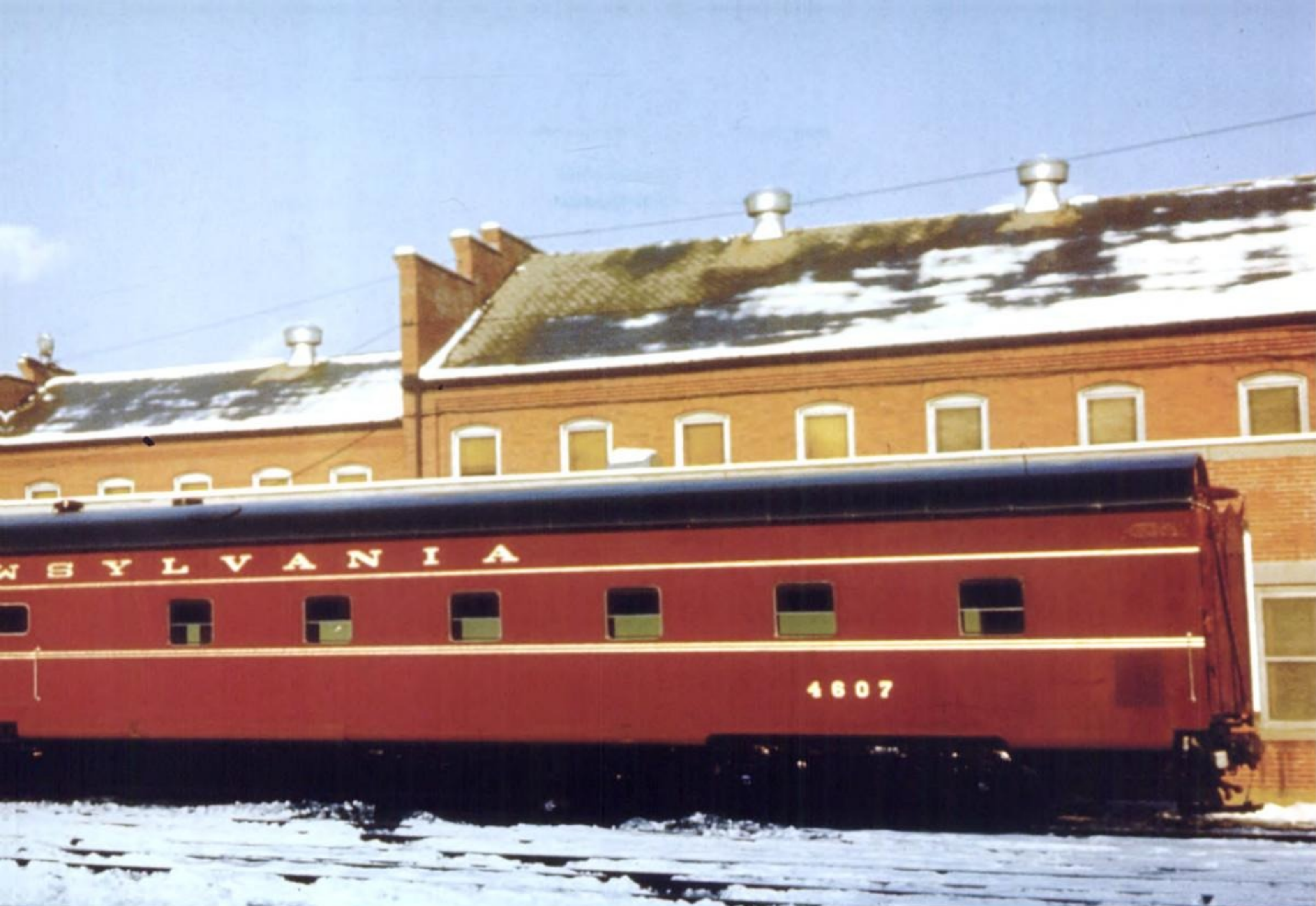
Dining car No. 4606 was paired with car No. 4607, which contained a kitchen and a dormitory for the dining car crew that rode all the way between endpoints. These cars, like the rest of the postwar Broadway Limited equipment, were finished in an attractive paint scheme of Tuscan Red and a black roof and underbody with gold lettering and striping. ACF archives, John W. Barriger III collection, St. Louis Mercantile Library, UMSL
